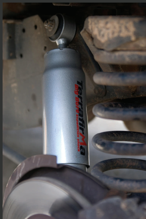
Below: The TerraFirma big bore shock fitted to the rear of my defender
